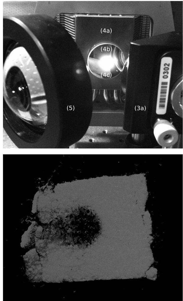
Figure 3: [Top] (4a) heat-sink with cooling fins and rear-mounted fan; (4b) protected aluminum mirror; (4c) Phosphor fluorescence under excitation by laser. [Bottom] YAG:Ce phosphor patch of dimensions approx.  $7 \text{ mm} \times 5 \text{ mm} \times 100 \mu\text{m}$  glued to mirror (4b.) Burn damage was due to hot spots from irregular modal distribution of laser diode when deformable mirror was inactive.
