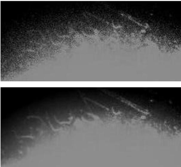
Figure 5: [Top] Emission and reflection from phosphor patch with deformable mirror inactive. Speckle arising from laser illumination is visible in the non-saturated periphery; [Bottom] With deformable mirror active state, speckle is not visible.
