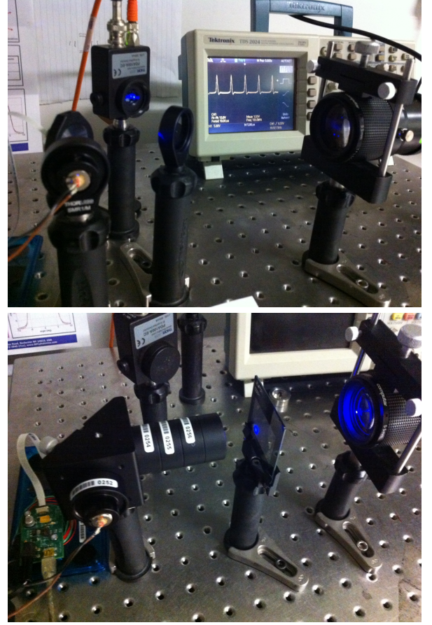
Figure 2: [Top] Apparatus to validate laser pulse duration: Nichia NDB7875 445 nm laser diode with collimating lens, deformable mirror, beamsplitter, photodiode, oscilloscope, and CCD camera. Roithner EU-38-TTL diode driver PCB and Agilent 33210A signal generator not shown. [Bottom] Apparatus to observe speckle in an acquired image: laser diode with 1\mu\text{s} pulses, low angle diffuser (stationary,) deformable mirror with a 380 kHz base actuation frequency, two low angle diffusers (stationary,) collector and condenser lenses and apertures in a Köhler configuration, neutral density filter, 10 mm diameter illumination on metal-on-glass Moire Grating (40 line pairs per mm,) camera with 6.45 \times 6.45 \mu\text{m}^2 CCD pixel size and approximately 1.5\times magnification through f=55\text{ mm} lens at aperture stop f/8 .
