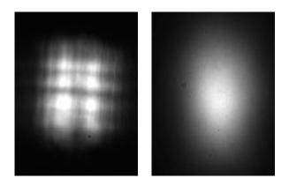
Figure 4: [Left] Thorlabs BC106-VIS beam profiler image of laser diode emission collimated and focused at infinity with simple lenses. Area is approximately  $1.5 \text{ mm} \times 1.0 \text{ mm}$ . Irregular intensity distribution is apparent. [Right] Beam profiler image of the same laser diode emission but reflected from the deformable mirror and focused with a positive lens into an area of similar size. To enhance visibility these images have different dynamic ranges.
