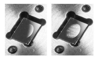
Figure 1: DYOPTYKA's miniaturized deformable mirror with elliptical active area of 3.0 mm by 4.5 mm and dielectric stack coating for high reflection efficiency. [Left] Deformable mirror inactive. [Right] Deformable mirror active, showing the randomly-distributed surface deformations which lead to the generation of uncorrelated speckle patterns.
