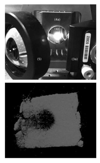
Figure 3: [Top] (4a) heat-sink with cooling fins and rear-mounted fan; (4b) protected aluminum mirror; (4c) Phosphor fluorescence under excitation by laser. [Bottom] YAG:Ce phosphor patch of dimensions approx.  $7 \text{ mm} \times 5 \text{ mm} \times 100 \text{ µm}$  glued to mirror (4b.) Burn damage was due to hot spots from irregular modal distribution of laser diode when deformable mirror was inactive.
