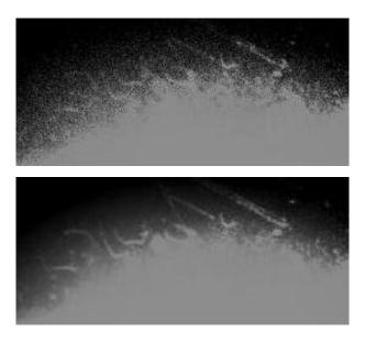
Figure 5: [Top] Emission and reflection from phosphor patch with deformable mirror inactive. Speckle arising from laser illumination is visible in the non-saturated periphery; [Bottom] With deformable mirror active state, speckle is not visible.
