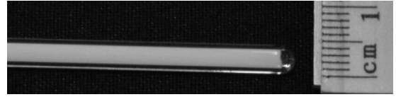
Figure 1: Strip of quantum dot materials encapsulated in a glass tube, from QD Vision, Inc.
