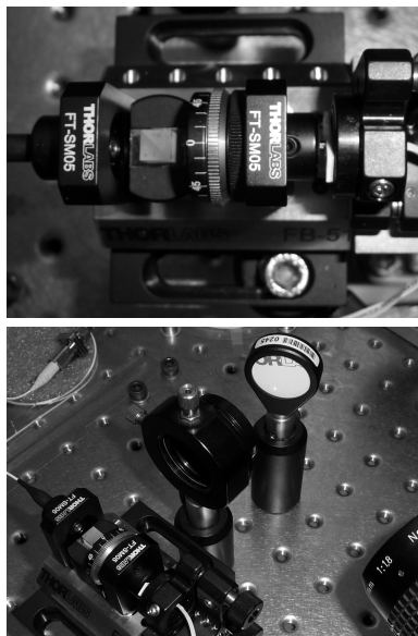
Fig. 3: [Top] Laboratory implementation of optical system shown in Figure 2: 635 nm laser delivered through single mode fiber with GRIN collimator for beam diameter of approx. 0.5 mm at 20 mm distance; polarizing beam splitter; achromatic quarter wave plate; GRIN focusing/collimating lens with 0.23 pitch and effective focal length of 1.85 mm; uDM2 deformable mirror; kinematic mount for precise alignment of uDM2. [Bottom] Additional components: 0.5 mm aperture-limiting stop in kinematic mount; smooth paper screen at approx. 115 mm from beam focusing/collimating lens; lens of camera for imaging of spot on screen.
