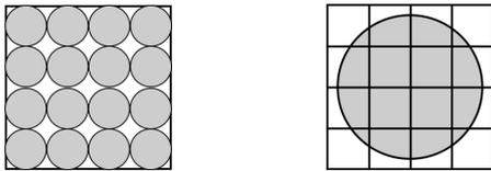
Fig. 5: [Left] When sensor pixel region on scattering surface is larger than the diffraction-limited spot size of the illumination optical system then minimum  $C_S = 1/\sqrt{n}$  for  $n$  spots [4]. [Right] In high-resolution imaging, sensor pixel regions are typically smaller which precludes spatial averaging of uncorrelated speckle patterns within the region for reduction of  $C_S$ .
