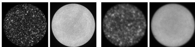
Fig. 1: Circular core; approx.  $26\times$  magnification of real image. [Left pair] Exit face; Deformable mirror inactive and active; Speckle contrast ratio  $C_S = 58.9\%$  and  $5.3\%$  respectively. [Right pair] Volume scatterer; Deformable mirror active and inactive;  $C_S = 28.9\%$  and  $5.8\%$  respectively. [Both pairs] With deformable mirror inactive, laser power was reduced to minimize sensor saturation by bright speckle grains.
