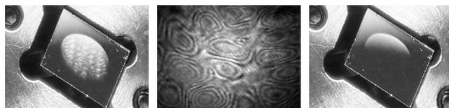
Fig. 3: [Left] Deformable mirror active. Randomly-distributed surface deformations are excited at very high frequencies in the  $3\text{ mm}\times 4.5\text{ mm}$  elliptical region. Reflectance  $\leq 99\%$  and damage threshold  $> 1\text{ Wmm}^{-2}$  for wavelength-appropriate mirror coatings. [Center] Microscope interferometer image showing fringes resulting from actual mirror deformations. [Right] Mirror inactive with near planar surface.
