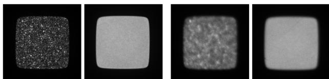
Fig. 2: Square core; approx.  $26\times$  magnification of real image. [Left pair] Exit face; Deformable mirror inactive and active;  $C_S = 47.5\%$  and  $3.6\%$  respectively. [Right pair] Volume scatterer; Deformable mirror active and inactive;  $C_S = 18.1\%$  and  $4.6\%$  respectively. [Both pairs] With deformable mirror inactive, laser power was reduced to minimize sensor saturation by bright speckle grains.
