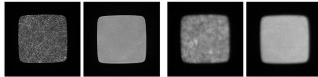
Fig. 7: Square core; approx.  $24\times$  magnification of real image. [Left pair] Exit face; Deformable mirror inactive and active;  $C_S = 31.9\%$  and  $3.8\%$  respectively. [Right pair] Volume scatterer; Deformable mirror active and inactive;  $C_S = 14.9\%$  and  $4.4\%$  respectively.
