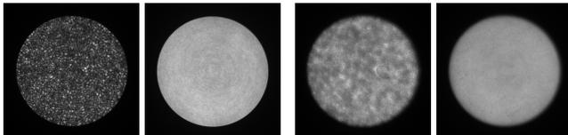
Fig. 6: Circular core; approx.  $24\times$  magnification of real image. [Left pair] Exit face; Deformable mirror inactive and active;  $C_S = 41.0\%$  and  $5.6\%$  respectively. [Right pair] Volume scatterer; Deformable mirror active and inactive;  $C_S = 16.8\%$  and  $5.2\%$  respectively.
