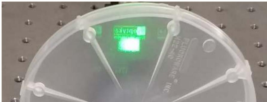
*PFA fluoropolymer, 2 mm thickness, smooth surface.*
