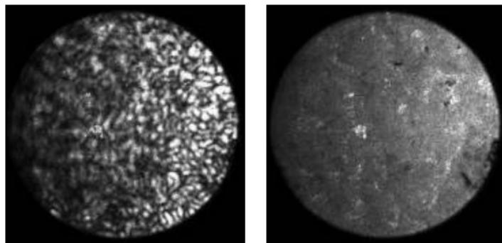
*Exit face of 105  $\mu\text{m}$  multimode fiber*
