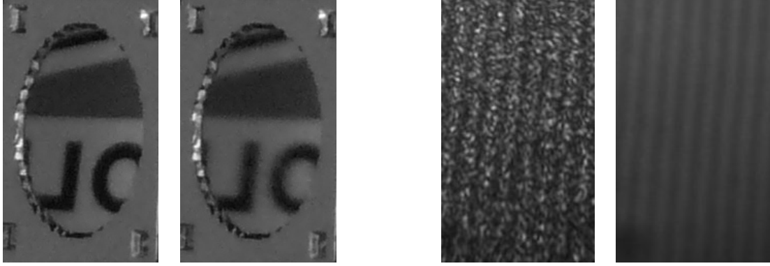
Figure 7. [Left] A deformable mirror prototype showing a reflection of some text when inactive and when active with approximately 0.5 degrees randomized divergence—showing the reflection blurred. [Right] Fringes from a Michelson interferometer with a deformable mirror in the common path before the split into two arms, when inactive and when active. These fringes demonstrate that beam directionality and coherence are preserved with the deformable mirror, i.e. it does not act as a diffuser to scatter illumination.
