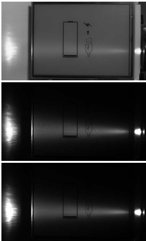
Fig. 3: Light Guide Plate illuminated by laser through multimode optical fiber. Camera lens f = 12.5 mm and f/11 . [Top] With additional broad spectrum incandescent bulb illumination of apparatus and 100 ms camera exposure period. [Middle] With laser illumination only, deformable mirror inactive, and 10 ms exposure period. [Bottom] As above but with deformable mirror active.
